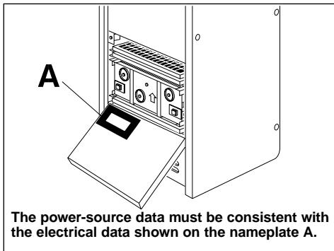
The power-source data must be consistent with the electrical data shown on the nameplate A.
